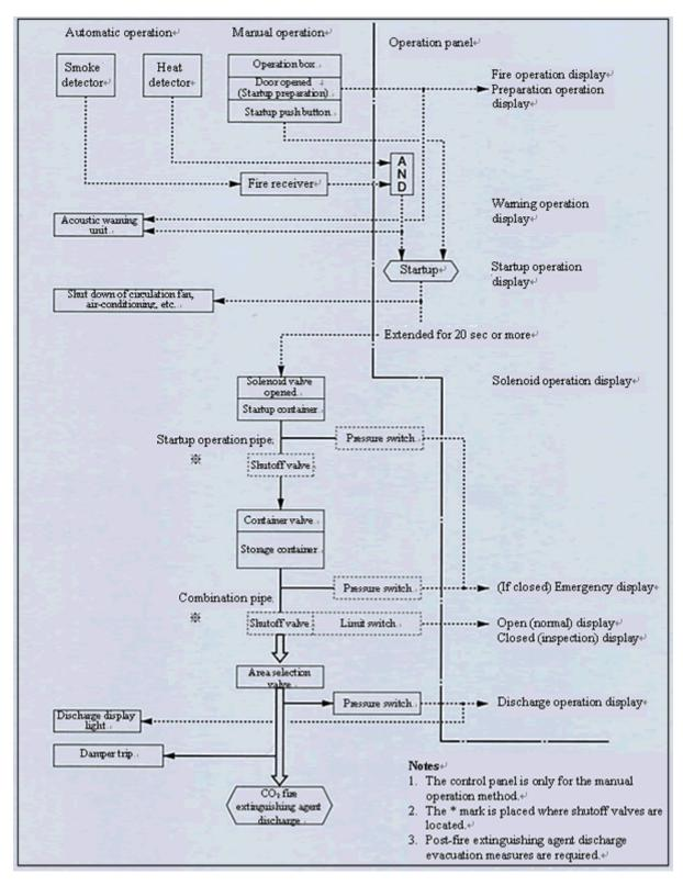
The carbon dioxide fire extinguishing system control panel, operation box, and shutoff valves comply with the technical standards for safety measures to prevent accidents to people from mistaken discharge and have been certified by the Japan Fire Equipment Safety Center. (Model No. NDC-CSS/Model No. System No. 007)
